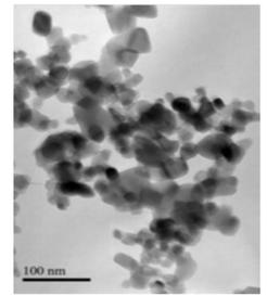
**Figure 1.** TEM image of Titanium Oxide (TiO<sub>2</sub>). These specific ENMs are used for exposures to both models. ENMs are from the European Commission's Joint Research Centre (JRC) and are standard particles used throughout the literature. <https://ec.europa.eu/jrc/en>
