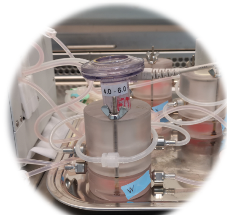
Figure 2. The assembled bioreactor connected to a perfusion system and an aerosol generator.
