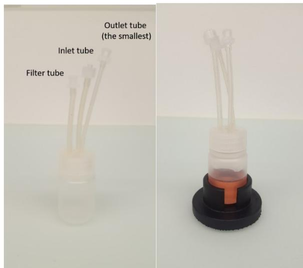
Figure 3 : Picture of the reservoir and its holder
