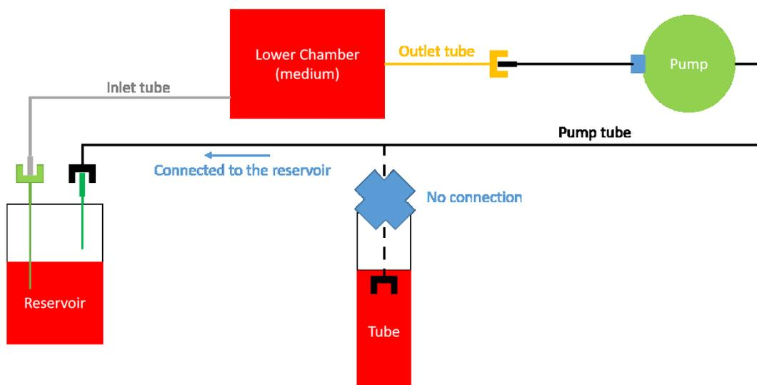
12. If the pump will go inside the incubator: move the pump, the reservoir and the bioreactor into the incubator, then skip to passage "15", otherwise:
