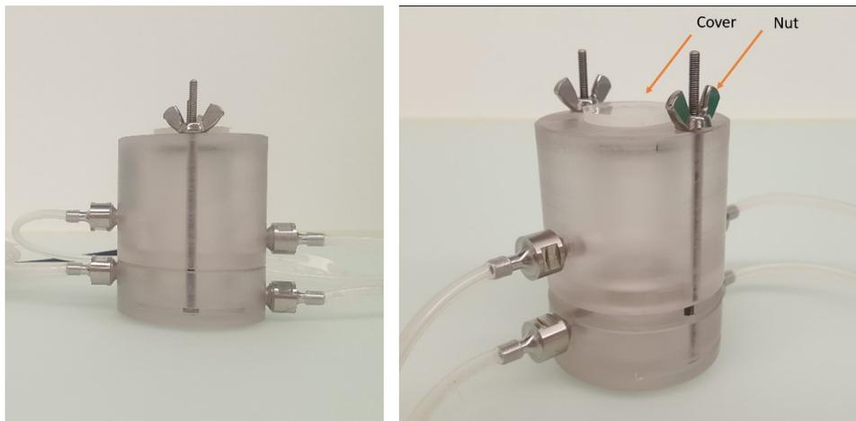
8. Turn the bioreactor → the inlet tube (the lower) must be on top (**important to avoid air bubbles formation in the lower chamber**)
