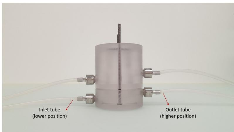
Figure 1 : Picture of the bioreactor
