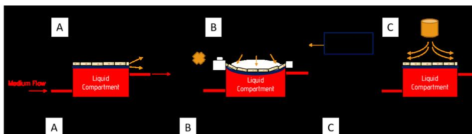
Figure 7: Key elements of the DALI system: A) ALI with media flow, B) stretching of the membrane and C) aerosol deposition on the cell layer.
