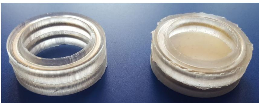
Figure 5 : Picture of the membrane holder
