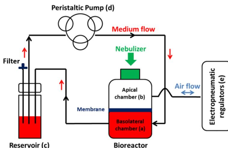
Figure 6: On the top: schematic view of the entire DALI system, which include a two-compartment bioreactor – (a) and (b) are respectively the basolateral and the apical chamber, a reservoir (c) from which the media is suck by a peristaltic pump (d), and a electropneumatic regulator (e) that introduce air in the upper chamber, allowing membrane stretching.
