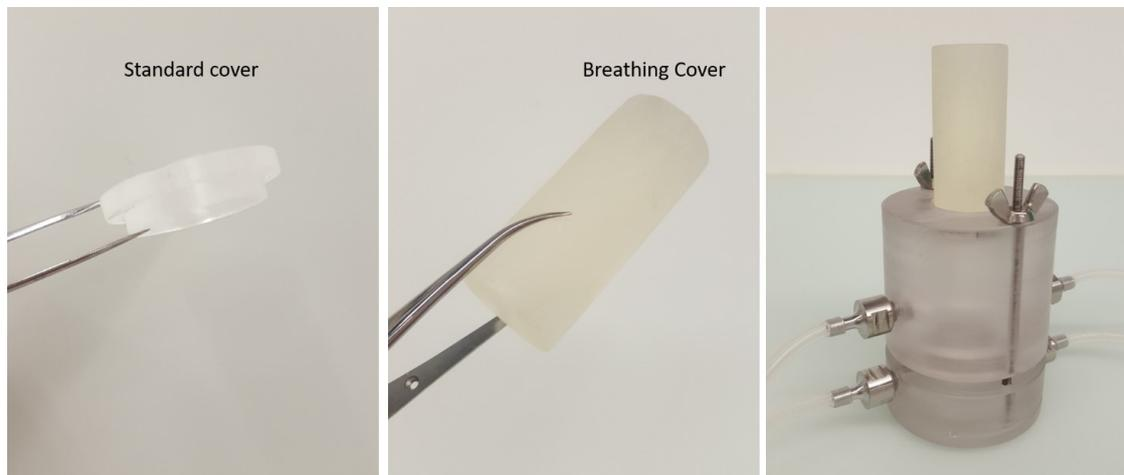
Figure 2 : Picture of the standard cover (to use without pressurization) and the breathing cover (to use during pressurization).
