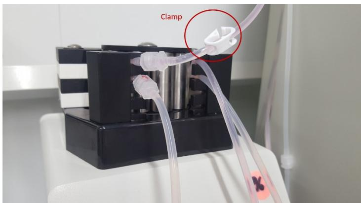
11. Reconnect the female end of the *pump tube* to the reservoir
