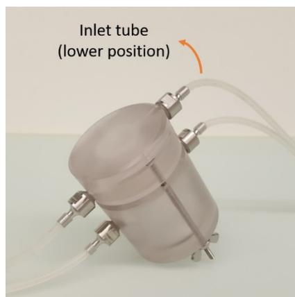
9. Disconnect the *pump tube* from the reservoir and put its female-end inside the tube with media. Start the pump (i.e. counterclockwise) and run it until the filling of the entire circuit.
