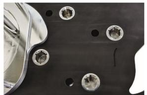
Figure 6 Base plate showing four microbalance positions replaced with four metal cups containing cell culture inserts.
