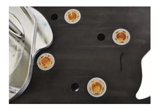
Figure 4 Baseplate showing all four microbalances in place.
