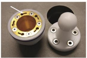
Figure 2 Microbalance assembly (left) and extraction tool (right) showing location holes (arrow) on the microbalance.
