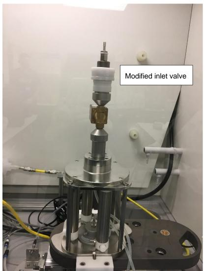
Figure 7 Final modification of the original exposure system. The modifications solved the issues related to deposition, however, to get the system into a usable format took more than 18 months from date of delivery.
